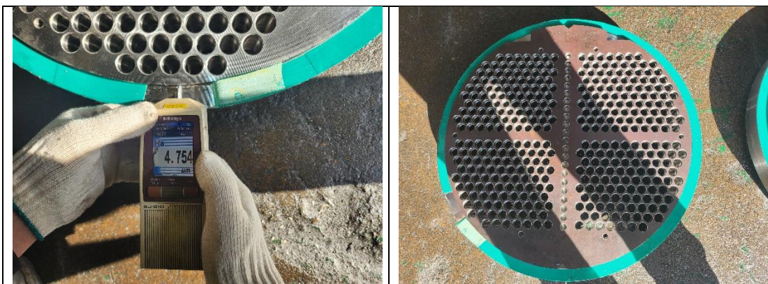
Tube Sheet: Visual Dimension, Marking Inspection
