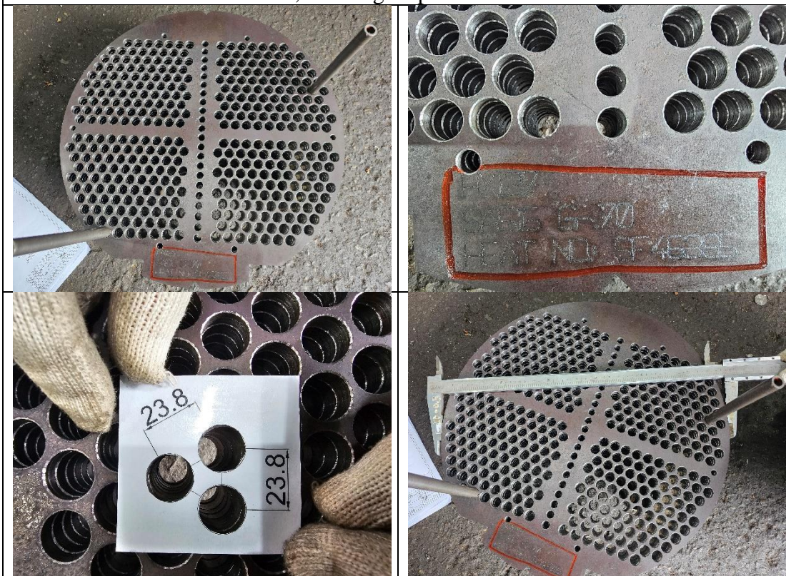
Tube Sheet: Visual Dimension, Marking Inspection
